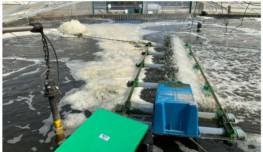
Endress+Hauser DO, pH and salinity Memosens® probes immersed within pond for online water quality monitoring.
