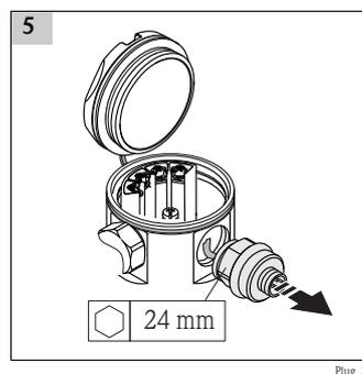
**Install plug M12 on sensor**
